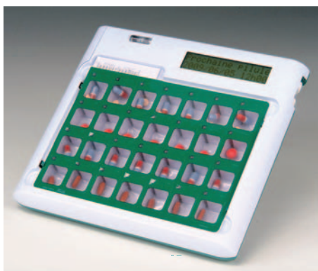
DO-Pill SecuR™: an intelligent electronic pill dispenser
